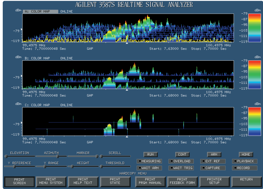
The color spectral map stacks multiple traces one on top of the other to show signal history with power shown as trace contours and color coding. Adjust azimuth to control apparent viewing angle (top). Adjust elevation to change vertical trace spacing (middle). Adjust threshold to emphasize signal peaks (bottom).
